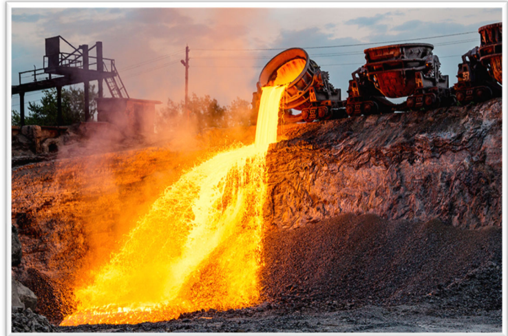
Figure 6-1. Iron slag being poured from slag pot.
