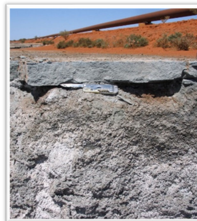
Heavily carbonated nickel mine tailings from the Mount Keith mine, Western Australia. 4
